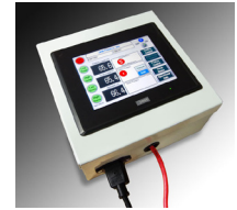
Remote Idec Control Panel
